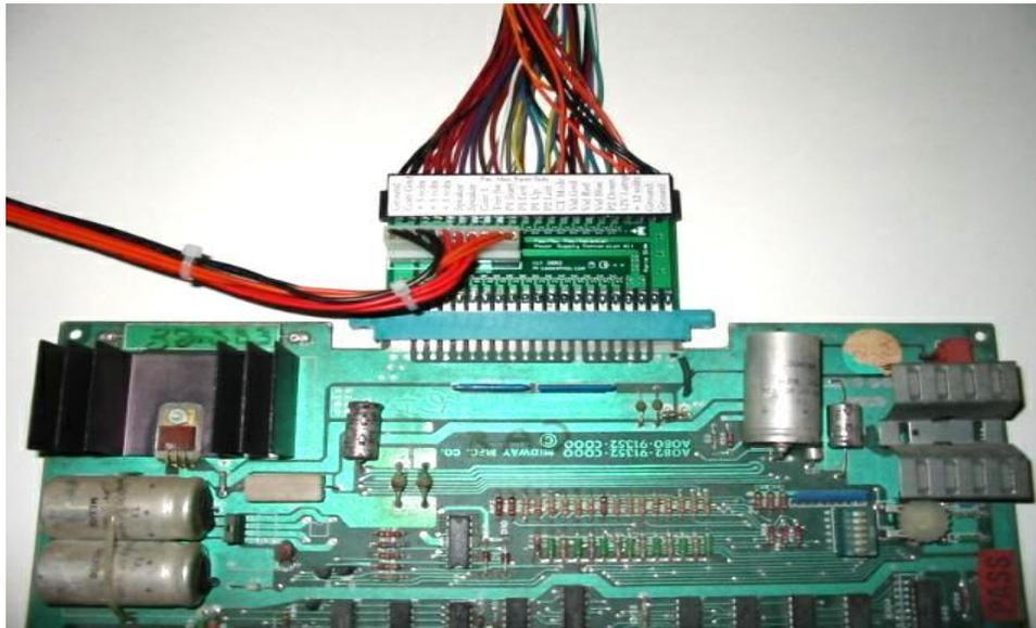
Locate the two A.C. power wires leading to the monitor. Find a convenient spot and tap the two A.C. wires from the new power supply to each of the monitor power wires.
