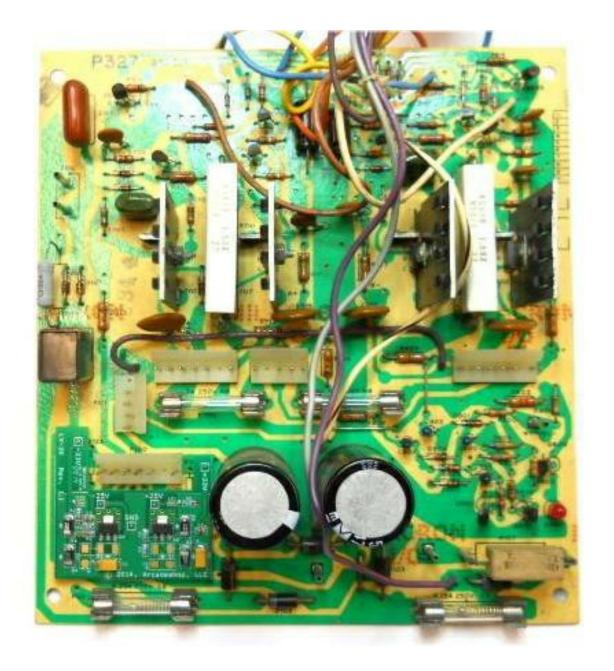
The LV-2K is optimally preset with output voltages of +/- 26v with a +/- 2% tolerance (25.48v to 26.52v) on each output.
