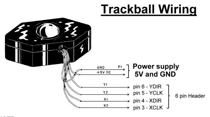
**NOTE:** boards before version "1.02 Rev.A" may require upgraded opto sensors in the trackball or spinner.
