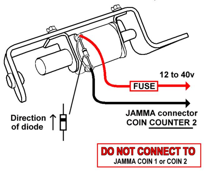
Two possible coils can be used **DEPENDING ON THE VOLTAGE USED!**
