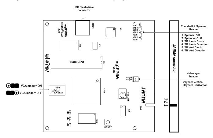
A six pin headers is provided on the board for Spinner and Trackball inputs. If the spinner or trackball is not used this header does not need to be connected.
